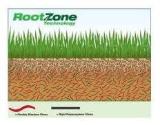
Fibrelastic is a similar alternative that aims to further improve the characteristics of typical fibre reinforced, sand-dominant rootzones by imparting a significant degree of resilience and energy absorption to the surface. This is achieved by mixing silica sand, organic matter, rigid polypropylene fibres and flexible elastane fibres to produce a completely homogeneous blend.
