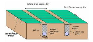
The costs of this maintenance regime will vary depending on levels of compaction, soil type and intensity of use, but would be around £30,000 per year for a 3ha site that already has a good quality drainage system installed, itself estimated to cost about £170k.
